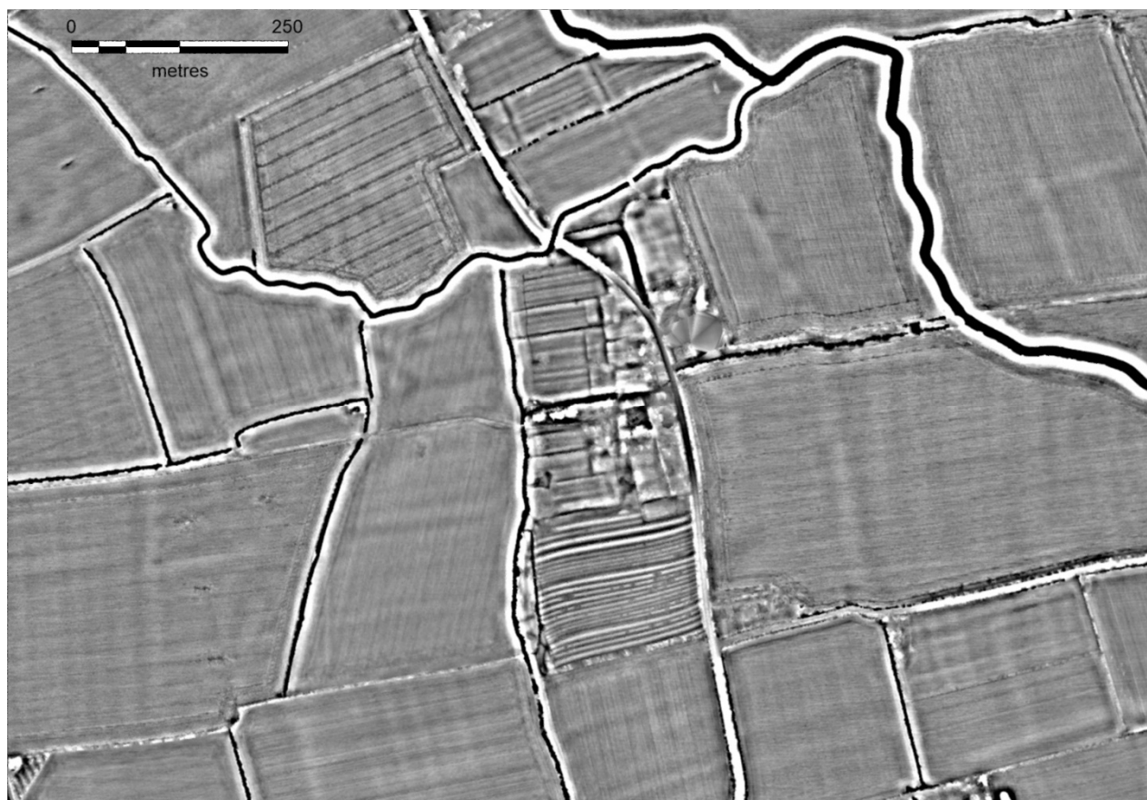
Figure B. Simple Local Relief Model (of DTM). General relief models convey landscape scale topography at the expense of smaller scale features including archaeological earthworks. This visualisation removes the general trend, eg hills and valleys to accentuate the appearance of the smaller scale features. In this visualisation the lighter tones represent banks and mounds, the darker, ditches and pits. This visualisation is particularly effective at revealing very low earthworks.
